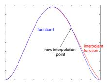
Figure 1: An Example of a *Local* Interpolation Method
