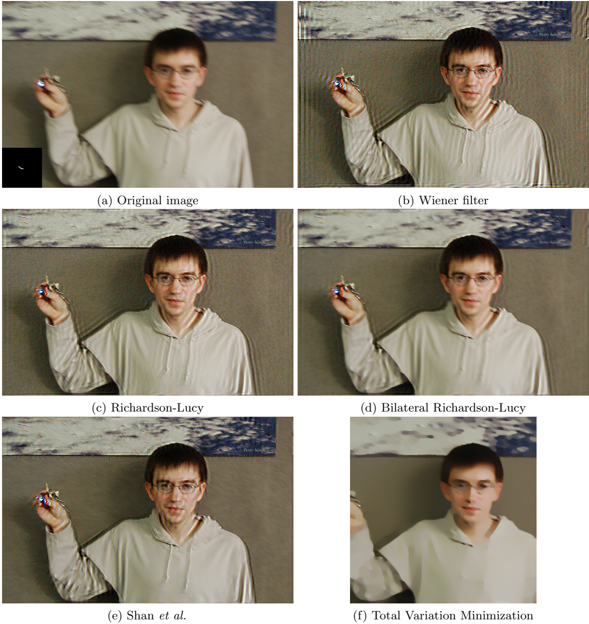
Figure 4: Shown above is the result of an experiment to manually estimate the blur kernel from a point light source in the original, blurry image. The blur kernel that we estimated is shown in the lower left corner of the original image (a). The Wiener filter result (b) contains the most ringing, following by the Richardson-Lucy result (c), Shan et al. 's result (e), the Bilateral Richardson-Lucy result (d), and finally the total variation minimization result (f). Total variation minimization tends to over smooth the result in regions of high variation. BRL performs well in this case, removing most of the ringing while still producing a crisp result.
