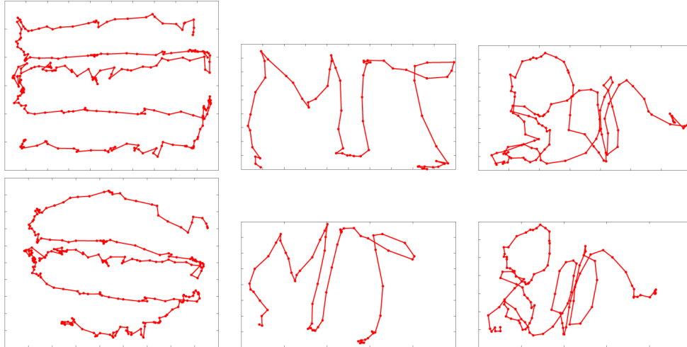
Figure 5-16: The top row is recovered using the supervised algorithm. The bottom row is recovered by the unsupervised algorithm. The middle panels is the recovered traces of someone writing "MIT." The right-most panels are the recovered traces of someone writing "Ben." The mapping recovered by the unsupervised algorithm is as useful for tracking human interaction as the mapping recovered by the fully calibrated regression algorithm.
