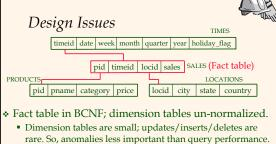
This kind of schema is very common in OLAP applications, and is called a star schema; computing
