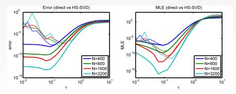
$y(\mathbf{x}) = sin(mean(\mathbf{x}))$ , using *N* Halton points solid lines for HS-SVD, dashed lines for direct solve
