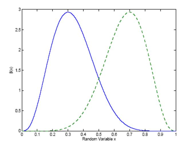
Figure 3. Beta distributions with a = 4 and b = 8 (solid line) and with a = 8 and b = 4 (dashed line). To get a higher peak (and stronger skew), use a and b that sum to a higher value.
