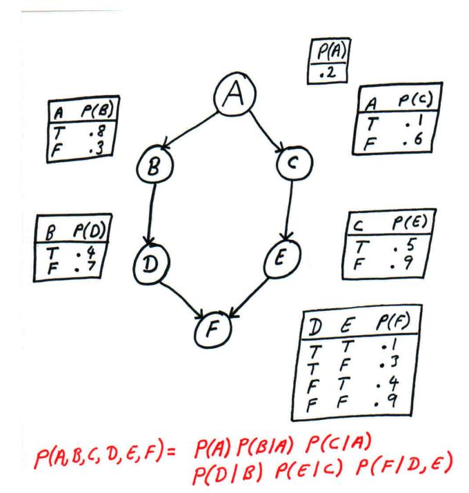
Query: P(F|C=true) Let's choose to eliminate in order A, B, C, D, E. 76 70 Before eliminating A, must multiply all potentials that involve A. JC C TC Eliminate A . 004 . 036 .144 .016 a by summing .224 ,336 if out. 096 .26 .34 .24 .16
