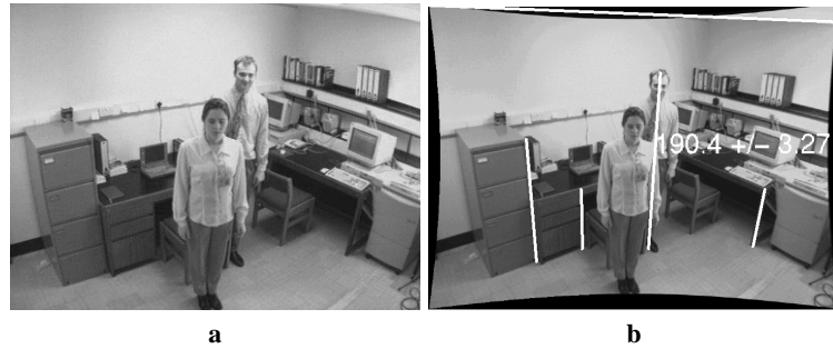
Fig. 10. Measuring heights of people from single views. (a) Original photograph. (b) Image corrected for radial distortion and measurements superimposed. Three reference heights (marked with white segments) have been used and the man height has been measured to be Z = 190.4 \pm 3.27 cm. The uncertainty on the measurements has been estimated according to [7].
