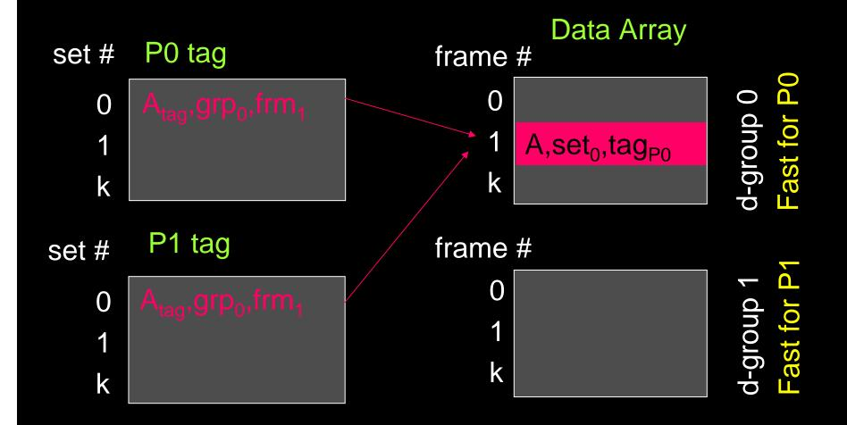
Supports controlled replication and in-situ communication
