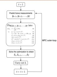
Predict future measurements, plan attack, carry out the current manipulation, and enter the next MPC iteration
