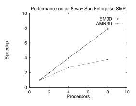
Figure 4: Speedups on an Sun Ultrasparc SMP
