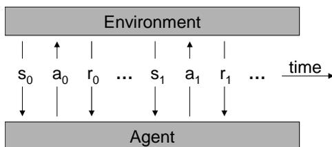
**Fig. 7.** A reinforcement learning agent interacts with its environment: it receives information about its state ( $s$ ), chooses an action to take ( $a$ ), receives a reward ( $r$ ), and then repeats.
