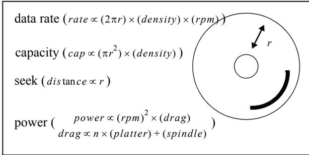
Figure 6: Diagram of basic drive parameters. A smaller media (lower  $r$ ) sacrifices bandwidth and capacity for shorter seeks and lower power. Each additional platter adds to capacity and power consumption.
