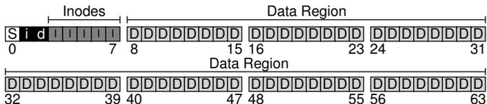
Thus, when mounting a file system, the operating system will read the superblock first, to initialize various parameters, and then attach the volume to the file-system tree. When files within the volume are accessed, the system will thus know exactly where to look for the needed on-disk structures.
