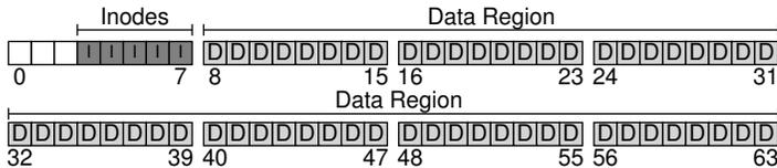
We should note here that inodes are typically not that big, for example 128 or 256 bytes. Assuming 256 bytes per inode, a 4-KB block can hold 16 inodes, and our file system above contains 80 total inodes. In our simple file system, built on a tiny 64-block partition, this number represents the maximum number of files we can have in our file system; however, do note that the same file system, built on a larger disk, could simply allocate a larger inode table and thus accommodate more files.
