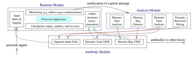
Figure 1: Architecture diagram of Sweeper
