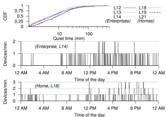
Figure 6: The plot shows (a) CDF of quiet times at locations where 48 hours of trace data was collected (enterprise and home locations). Time-series of non-WiFi device instances per minute at (b) an enterprise (location L14) and (c) and home (location L18) for a 24 hour period shows increased quiet times during late nights.
