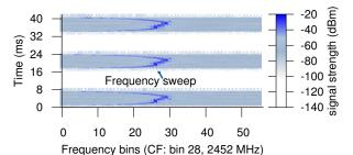
Figure 13: Spectral samples from Airshark capturing the activity of a residential microwave. The plot shows (i) the ON-OFF cycle for is around  $16.6~\mathrm{ms}$  and (ii) "frequency sweeps" during the ON periods.
