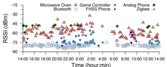
Figure 2: Average RSSI from different non-WiFi RF device instances shown against the device start times. Measurements were taken at a dorm-style apartment (location L16, dataset §2) for a 24 hour period.
