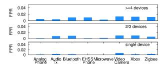
Figure 17: False positive rate for different devices.
