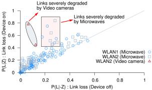
Figure 21: Results from a two day deployment of Airshark in two production WLANs. Each point in the scatter plot denotes the loss rate for a link in the absence  $(p(L|\neg Z))$  and the loss rate in the presence (p(L|Z)) of (i) microwave ovens, (ii) video cameras, for a total of 224 links (168 links in WLAN1 and 56 links in WLAN2).
