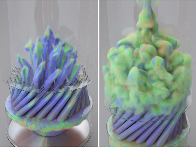
Figure 5: Smoke injected from the bottom of a cylinder, and forced through a twisted bundle of cylindrical holes. Color corresponds to vorticity magnitude. Total 1.2B active cells, in a 1024^2 \times 2048 grid.
