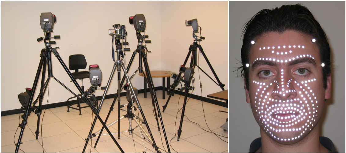
Figure 5.2: Eight camera, 250 marker optical motion capture layout
