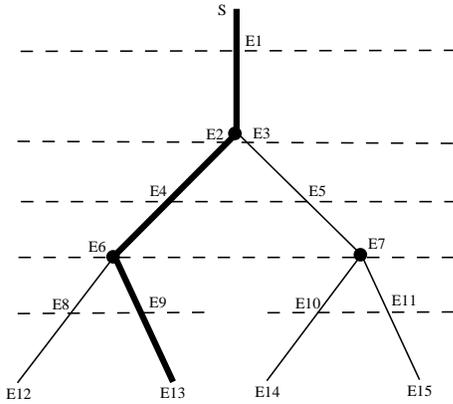
Fig. 12. OPB-UP Segment Partitioning for an Example Media Structure (“S” label is for start of media, “Ei” labels are for segment end points, dashed lines indicate segment boundaries,  $K = 6$ ,  $s = 2$ ,  $r = 1$ )
