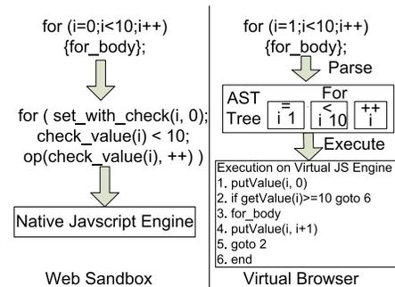
Figure 2: Comparison of Web Sandbox and Virtual Browser when Executing For-loop
