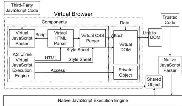
Figure 5: System Architecture
