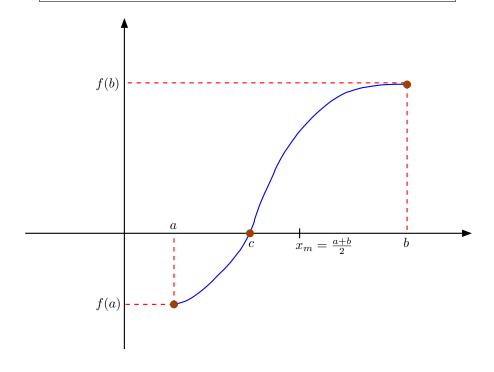
The bisection algorithm attempts to locate the value c where the graph of f crosses over zero, by checking whether it belongs to either of the two sub-intervals  $[a, x_m]$ ,  $[x_m, b]$ , where  $x_m$  is the midpoint
