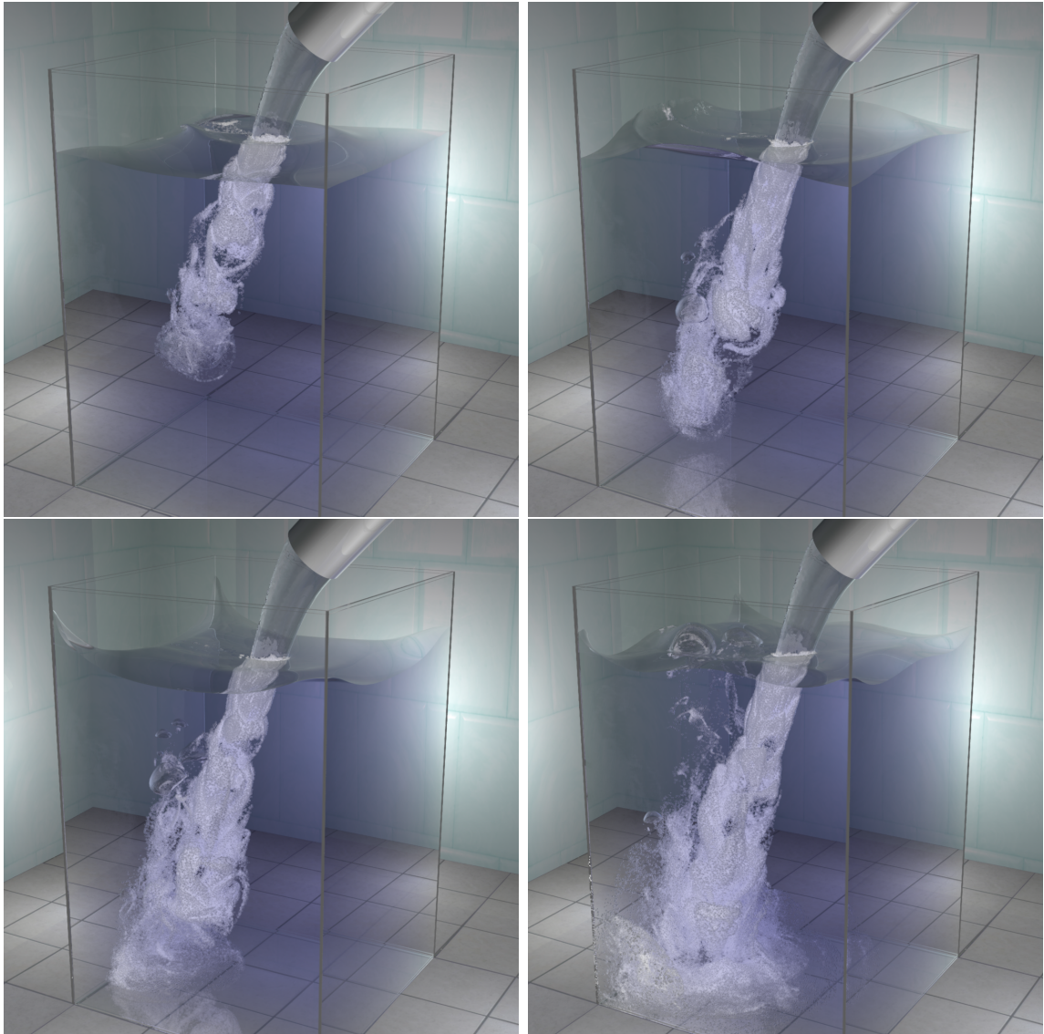
Figure 10.4: Faucet pouring water showing air entrainment ( 200 \times 400 \times 200 grid); about 300,000 sub-grid bubbles. Note that the size of the sub-grid bubbles was accentuated to highlight the complex bubble interactions and the dynamic flow field.
