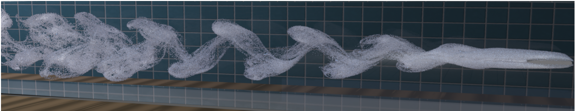
Figure 10.2: A fast moving hydrofoil generates the typical Von Karman vortex street in its wake through cavitation. The vortex street is generated because of the two-dimensional cross-sectional nature of the hydrofoil ( 1024 \times 128 \times 128 grid); about 600,000 sub-grid bubbles.
