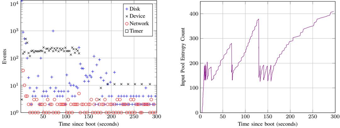
Figure 4. **(Left)** The number of event descriptions input to `/dev/(u)random` RNG by type of system event for the first 5 minutes of boot captured on VMware. The y-axis contains number of events (logscale) that occurred during each 3-second bin. **(Right)** The value of the input pool’s entropy counter `IP.ec` during boot.
