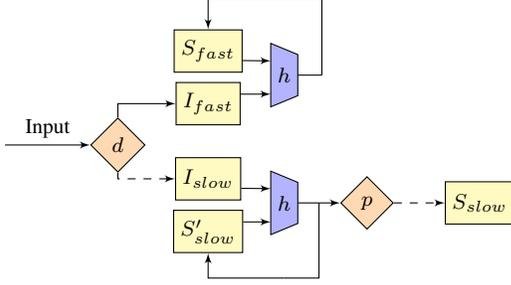
Figure 9. Block diagram of the Whirlwind RNG. Every  $d^{\text{th}}$  input is directed to the slow pool, and after  $p$  updates it is for use in output generation. Here  $h$  is the SHA-512 compression function.
