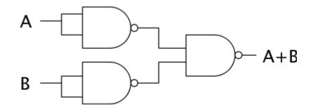
d) Make a NOR gate from only NAND gates (use <u>exactly</u> 4 NAND gates)
