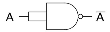
b) Make an AND gate from only NAND gates (use <u>exactly</u> 2 NAND gates)
