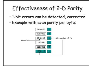
• 2-bit errors can also be detected
