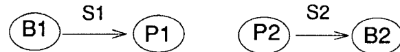
Figure 7: A two cell configuration where both pads are in range of their respective base stations and also in range of each other. Base station B1 is sending data to pad P1, and pad P2 is sending data to base station B2. Each stream is generating data at a rate of 64 packets per second and using UDP for transport.
