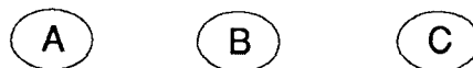
Figure 1: Station B can hear both A and C, but A and C cannot hear each other. A "hidden terminal" scenario results when C attempts to transmit while A is transmitting to B. An "exposed terminal" scenario results if B is transmitting to A when C attempts to transmit.
