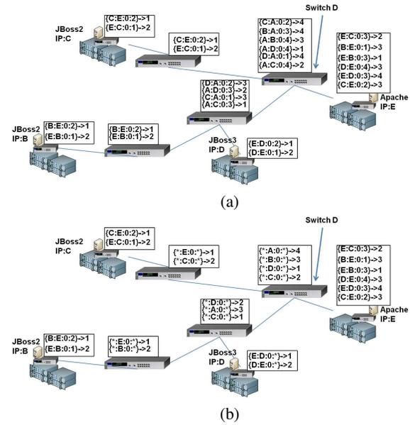
**Figure 5: A network with 4 hosts, 4 switches, and 4 VMs. The flow table for each switch is displayed in a white rectangle. The flow entries in each table have the following format: {Src IP:Dest IP:ToS:InPort}-> OutPort with a \* indicating a wildcard.**
