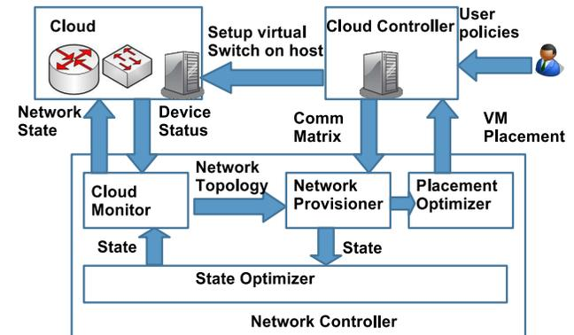
**Figure 4: Internal components of the network controller.**
