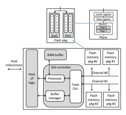
Figure 1: SSD internal architecture
