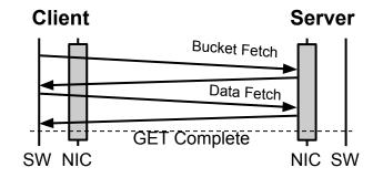
A 2xR-style R=1 Lookup operation using RMA primitives. A first operation to a predictable location *finds* the datum in an index. A second, dependent operation *retrieves* the datum.
