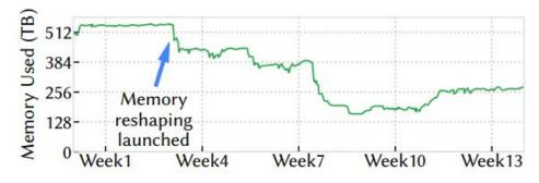
Plot of memory usage over time after *Dynamic Backend Scaling*'s initial rollout. Initially, capacity was simply slightly overprovisioned - this memory could be released. At ~Week 8, demand on corpus fell and more memory could be safely refunded.
