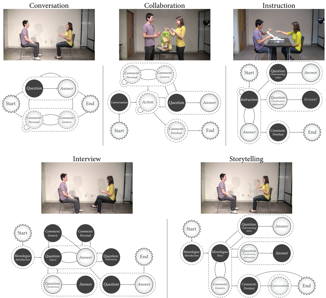
Figure 2. Five hand-crafted HRI templates derived from dyadic human-human interaction data. Each template contains a start and an end state. Dark and light gray states represent one or other agent in the dyad, respectively. States with dotted outlines can be enacted by either agent. Larger dotted regions correspond to the patterns uncovered by Sauppé & Mutlu [17].
