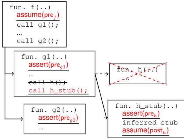
Fig. 3. A schematic illustration of depth cutoff in DC2 on a call graph.
