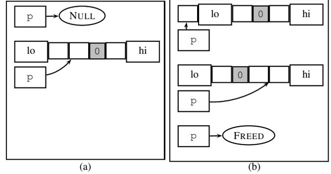
Fig. 5. Possible pointer configurations of an input string `p`: (a) part of default assumptions, and (b) not permitted by the default assumptions.
