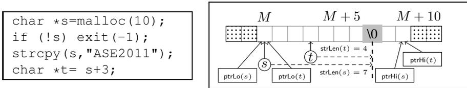
Fig. 1. The memory model for the array bounds model after successfully executing the four statements on the left-hand side: The successful allocation returns a pointer to some new address  $M$ , and the lower bound addresses  $\text{ptrLo}(s) = \text{ptrLo}(t) = M$ . The higher bound addresses are  $\text{ptrHi}(s) = \text{ptrHi}(t) = M+9$ . Finally, the string lengths are determined using the size abstraction, namely  $\text{strLen}(s) = 7$  and  $\text{strLen}(t) = 4$ .
