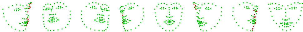
Figure 1: The modal viewpoints found for V = 8 viewpoint domains. The modal occlusion state of the landmarks is stored for each viewpoint domain (green is visible, red is occluded). Features are extracted around only visible landmarks.
