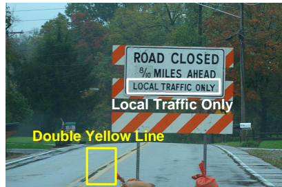
Figure 1: A fully self-driving system may fail to recognize the semantic meaning of “local traffic” and crossing double yellow line is allowed.
