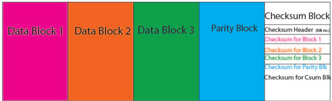
Figure 1: Our Checksumming RAID Layout. We have added another block to a typical RAID stripe to hold checksum data. The checksum block has a header which includes the block number, followed by a number of checksum entries indexed by the disk number, including one for itself.
