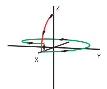
Figure 5-1: The idea behind unitary correction. Suppose we want to keep the Bloch vector in the x-y-plane. We first rotate the vector into the x-y-plane (the red path). The vector spins about the z-axis and relaxes (the green path). Then we try to push it back into the x-y-plane (the orange path). Such a procedure will result in a steady state Bloch vector.
