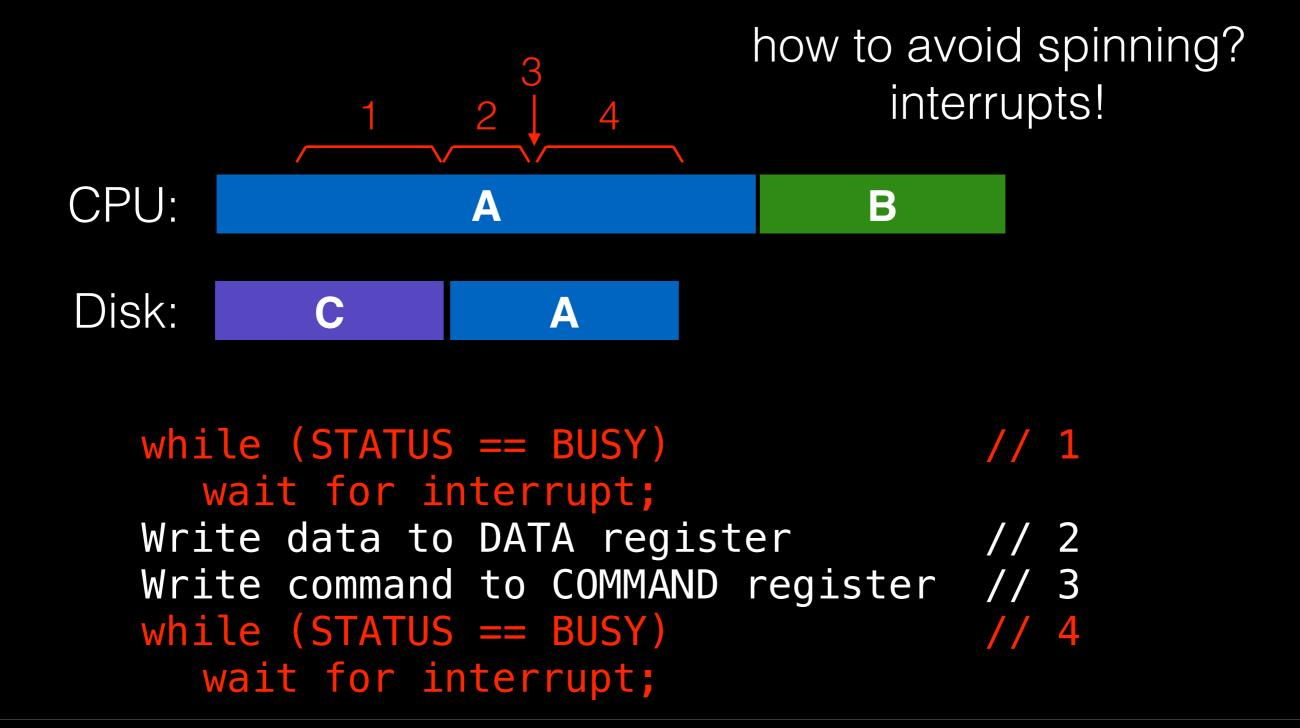
how to avoid spinning? interrupts! CPU: B A A Disk: C A while (STATUS == BUSY) wait for interrupt; Write data to DATA register Write command to COMMAND register // 3 // 4 while (STATUS == BUSY) wait for interrupt;
