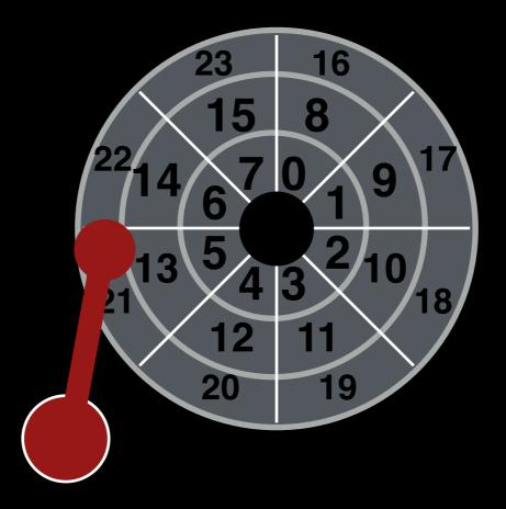
Heads on a moving arm can read from each surface.
