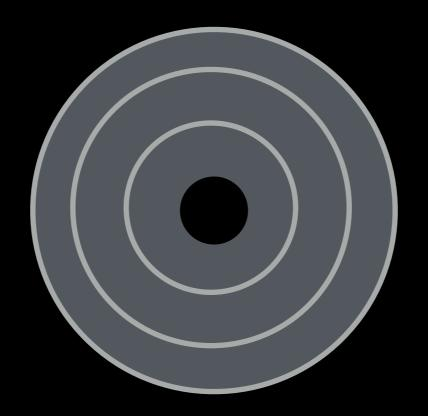
Each surface is divided into rings called <u>tracks</u>. A stack of tracks (across platters) is called a <u>cylinder</u>.
