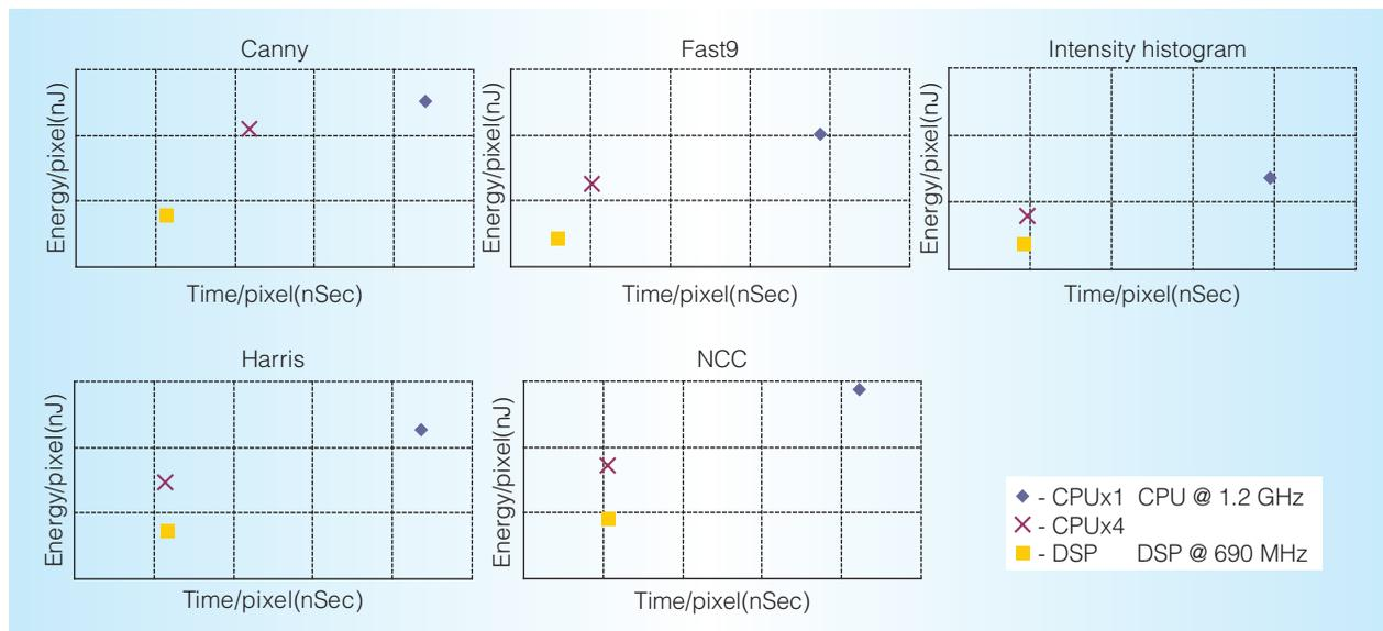
Figure 11. Energy versus latency for multimedia benchmarks. Each chart features a different algorithm used in a computer vision application.
