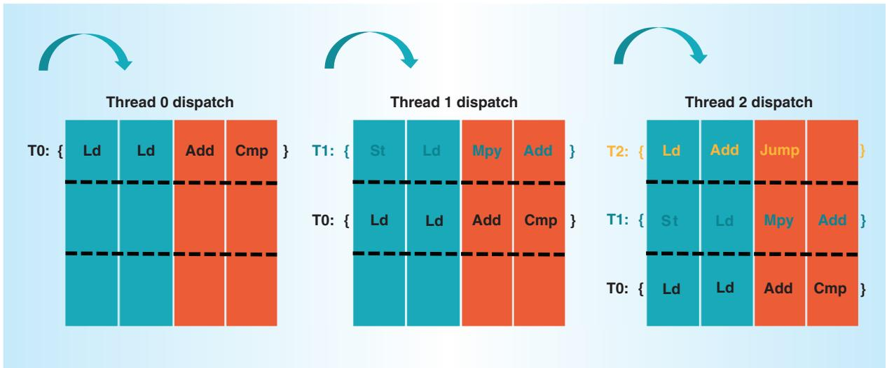
Figure 7. Interleaved multithreading. The figure shows a three-stage execution pipeline with three threads taking turns dispatching packets.
