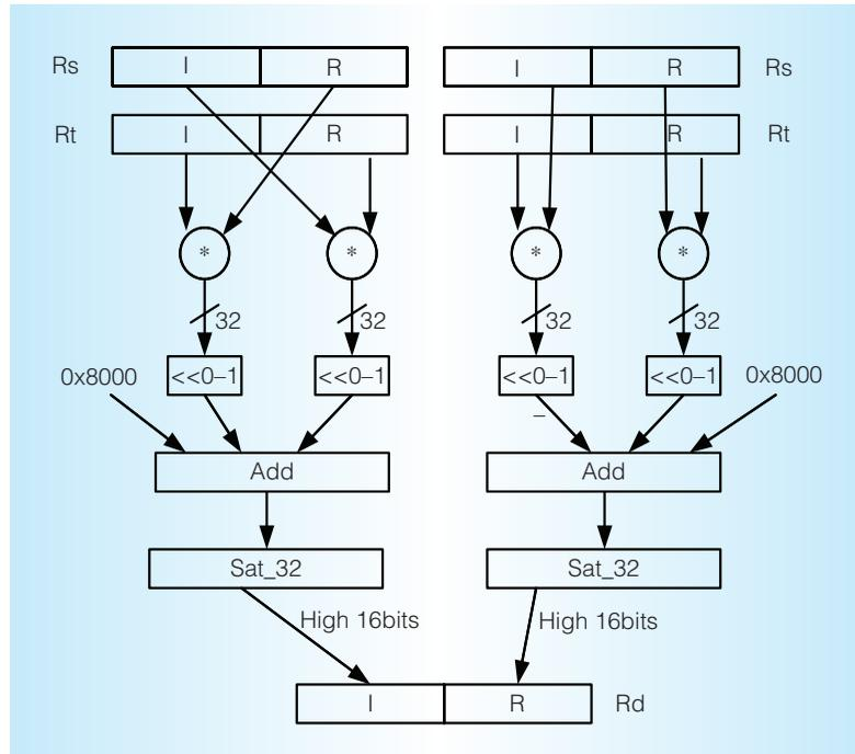
Figure 4. Complex multiply instruction. Such an instruction executed in a single pipelined execution unit provides large efficiency gains for applications that use complex arithmetic.
