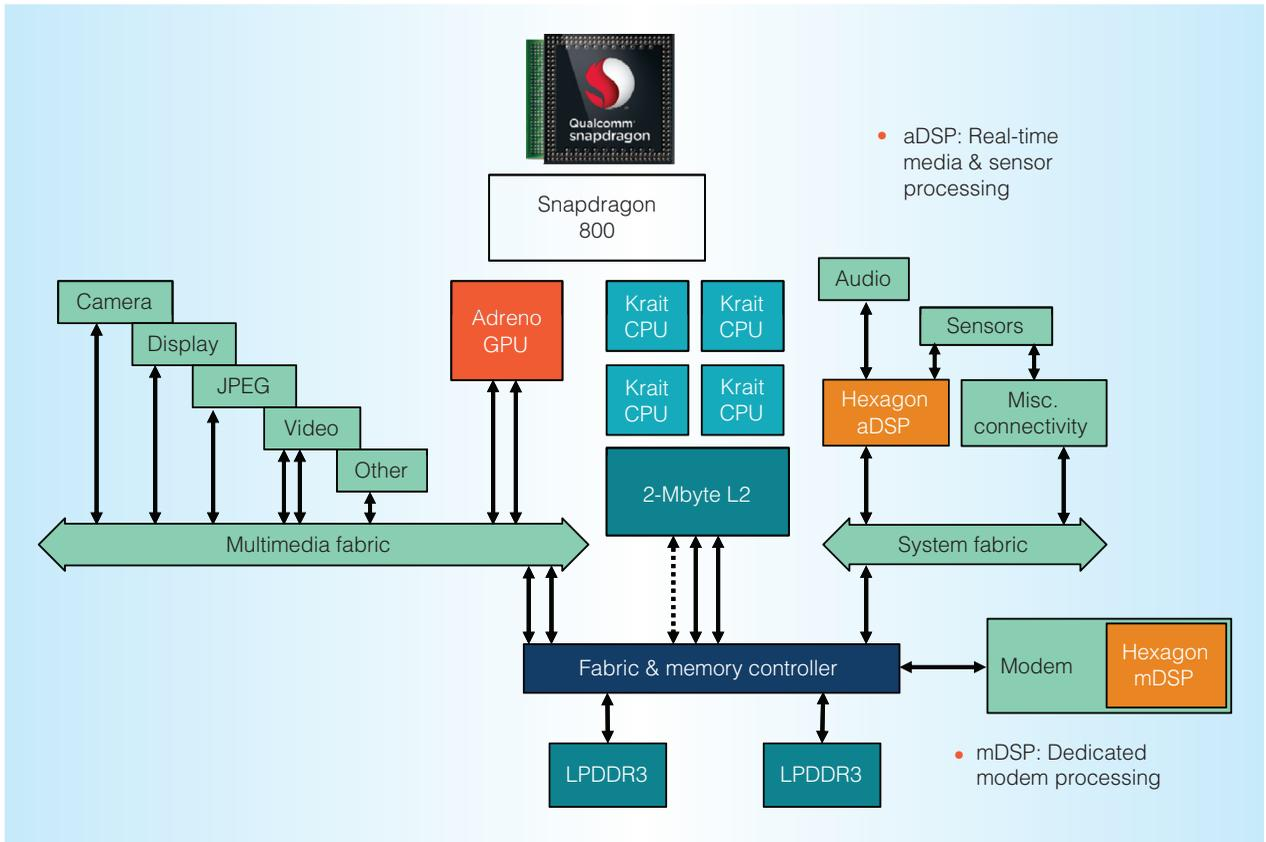
Figure 1. Snapdragon 800 block diagram. The chip contains dedicated subsystems for camera, display, video, audio/voice, sensors, graphics, cellular modem, and Wi-Fi.
