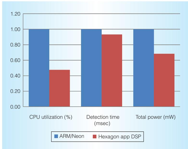
Figure 10. An example of feature detection offload. The algorithm is offloaded from the CPU to DSP, which results in comparable performance but much reduced battery current.
