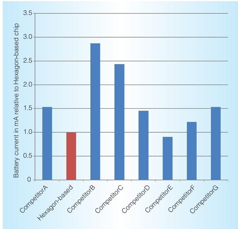
Figure 9. MP3 playback battery current for various smartphones. Lower bars represent more hours of music playback, which is a critical customer metric.
