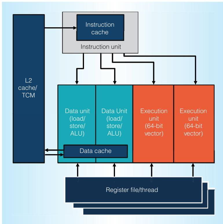
Figure 3. Hexagon block diagram. The architecture features a four-wide very long instruction word (VLIW) with dual load/store and dual single-instruction, multiple-data (SIMD) execution units and supports hardware multithreading.
