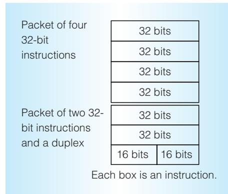
Figure 5. Visualization of a duplex. A duplex is a 32-bit subpacket containing two 16-bit instructions.
