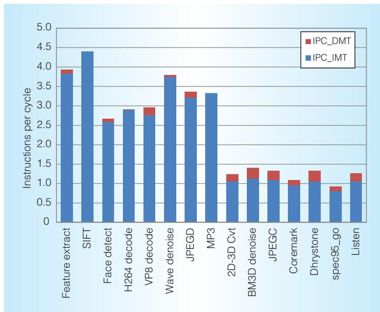
Figure 8. Performance on multimedia applications. The figure shows the instructions per cycle (IPCs) for various multimedia benchmarks, which are sorted into multithreaded applications (left) and single-threaded applications (right).
