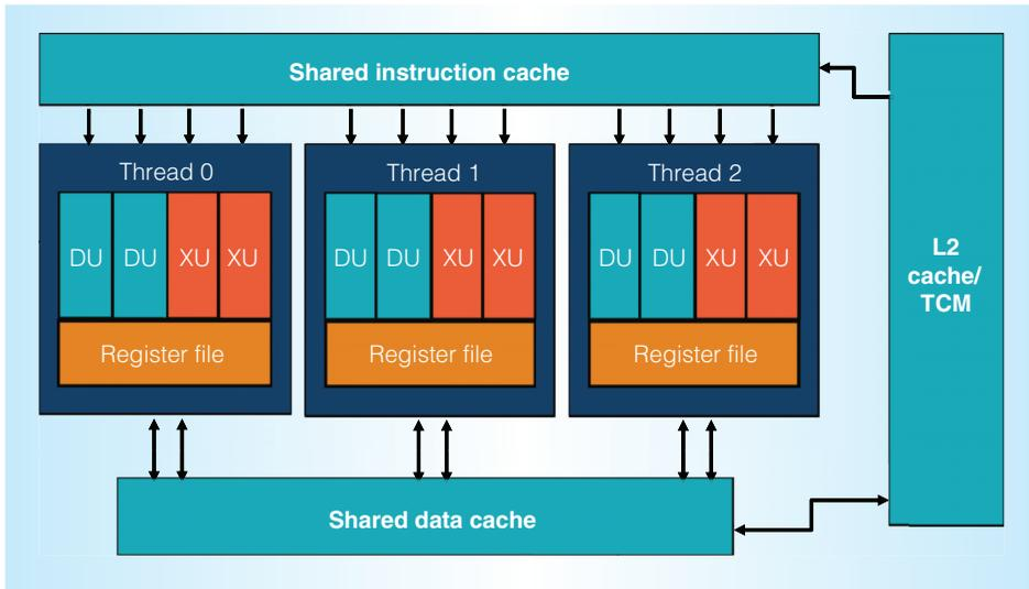
Figure 6. The programmer's view of multithreading. To the programmer, it appears as three VLIW cores with shared caches. Software threads are mapped to hardware threads by the Hexagon operating system.
