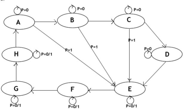
We add a new input P corresponding to the Pedestrian button. If vehicle light is green, (states A ,B ,C ,D) the state changes to amber (state E) if the button is pressed. In all other cases the button is ignored.
