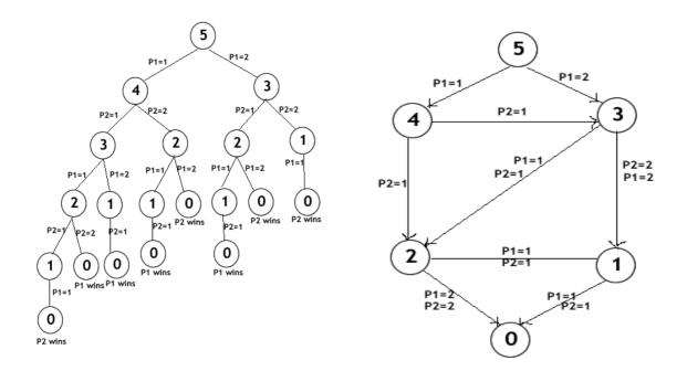
Each state corresponds to the number of balls left in the pile. The game is over when all the balls are gone, i.e. state is '0'. Each transition is labeled by player's choice: P1=1 means Player 1 picked 1 ball from the pile.
