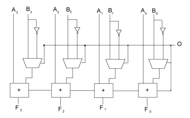
When O is 0, the MUXes choose the B inputs directly so the sum obtained is (A+B). When O is 1, the MUXes choose the negated bits of B (i.e. 1's complement of B). Also the carry-in of the left most adder is set to 1, the net effect of which is that the 2's complement of B is computed, and the result is A+(-B)=A-B.
