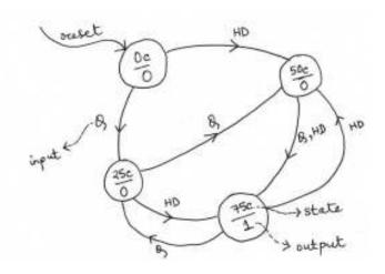
II. How many flip-flops (storage elements) will be needed to implement this finite state machine designed in your answer to part I?
