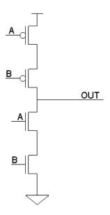
The output OUT is neither connected to Power not Ground when either A = 1 and B = 0 or A = 0 and B = 1, thereby creating an open circuit.
