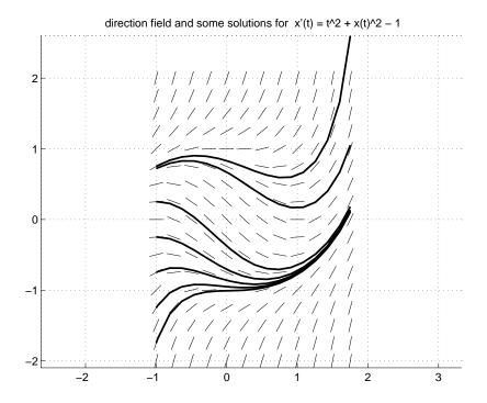
The figure shows, at various points in the (t, z)-plane, a little line segment whose slope equals f(t, z). If (t, z) is one of these points, and the solution of interest to us has the value z at t, i.e., y(t) = z, then its graph would go through the point (t, z) with slope exactly that of the little line segment plotted there.
