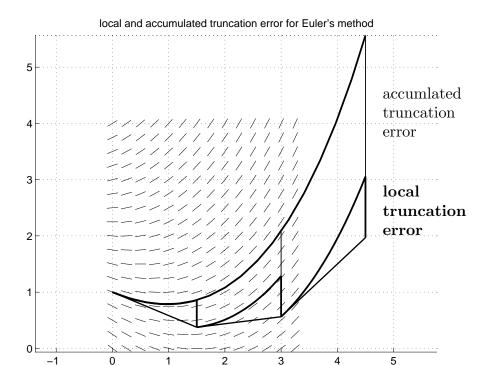
The details of such a **step-size control** can be quite intricate, but the basic idea is simple: after taking a step of size h, compare an estimate for the local truncation error with a specified tolerance; if the tolerance is smaller, shorten (usually, halve) the step size and try again; if the tolerance is slightly larger, accept and do the next step with the same h; if the tolerance is significantly larger, accept and do the next step with a larger (usually, doubled) h.
