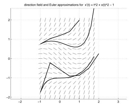
For the upper solution, the last two steps of Euler's method aren't even shown since it has a value greater than 12 by the time it reaches t=2. For the lower solution, Euler's method also initially grows much faster, but is then pushed back by those negative slopes and ultimately seems to parallel the correct solution, at a slightly lower level.
