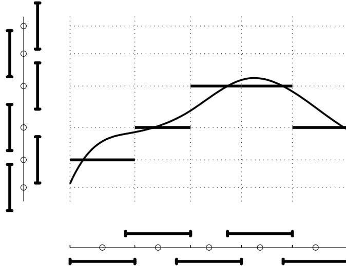
(39) Figure. An  $r$ -net for a totally bounded set of functions.
