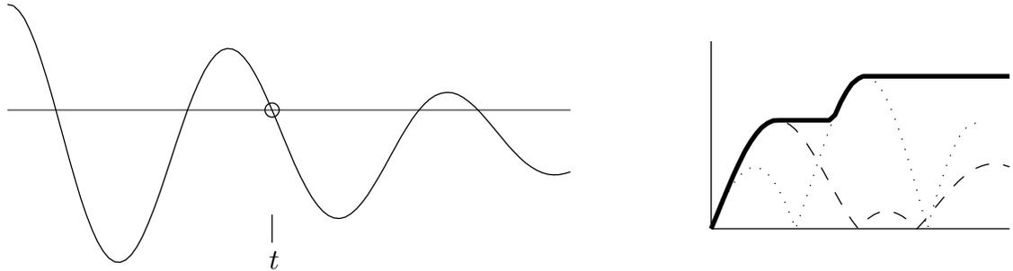
(12) Figure. Construction of  $\omega_{f,t}$  (heavy) as the ‘sunrise function’  $h \mapsto \max\{f_r(s), f_l(s) : s \leq h\}$  of  $f_r : h \mapsto |f(t+h) - f(t)|$  (dashed) and  $f_l : h \mapsto |f(t-h) - f(t)|$  (dotted).
