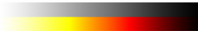
Figure 3.4.1: The black body palette, a widely used approximation for the light perceived from carbon-based combustion. Figure borrowed from Nielsen [8].
