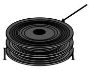
Old FS: All super-block copies are on the top platter Correlated failures! What if top platter dies?
