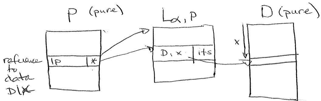
linkage section is different for every process
