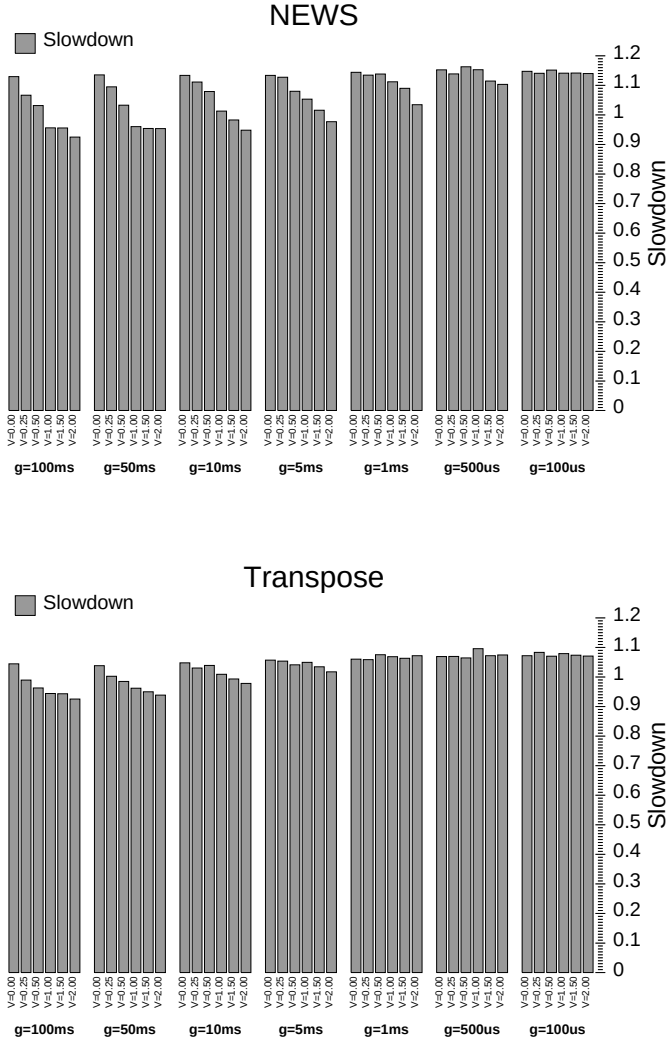
Figure 10.2: Performance on Bulk-Synchronous Workloads. The graphs compare implicit coscheduling with the full conditional two-phase waiting algorithm (i.e., baseline and conditional spin amounts as specified in Table 9.2) to ideal explicit coscheduling with spin-waiting. The workload consists of three bulk-synchronous jobs on 16 workstations. Both the NEWS and Transpose communication patterns are examined; in each case, the time between read operations is fixed at c = 8\mu s . The time between barriers, g , is varied between 100\mu s and 100ms across the sets of bars. Within each set of bars, the load-imbalance across processes is varied from V = 0 to V = 2 \cdot g .
