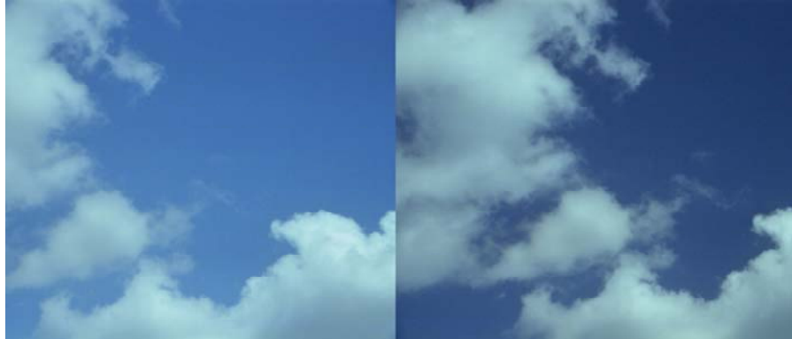
w/o polarizer w/ polarizer the filter darkens the cloud by about 1/2, but darkens the sky even more
