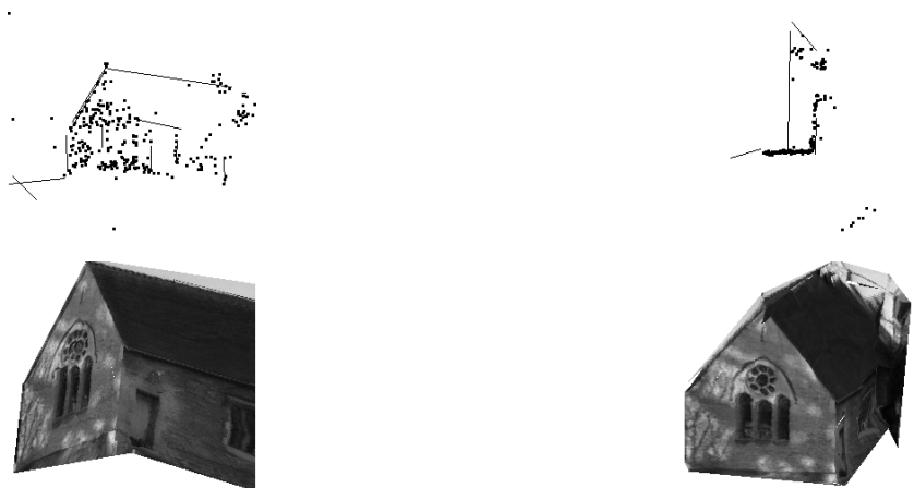
Figure 7: Results for the outdoor scene of a chapel of Figure 2. Details are as for the previous figure. The top-right figure shows a plan view of the recovered structure (perpendicular lines at upper-left) and camera positions (arc at lower-right). The camera positions lie at irregular intervals along a rough arc, which is a true reflection of the motion - the sequence was taken with a hand-held camcorder and the motion was not smooth. The dappling effect on the front of the chapel is sunshine through trees.
