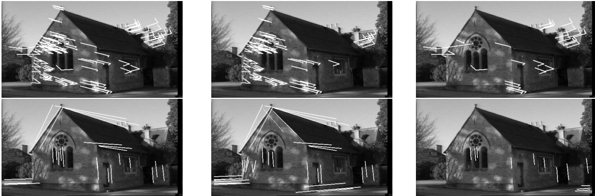
Figure 4: Results for matching a triplet of images using the trifocal tensor, superimposed onto the last image. Top (left to right) left : point correspondences over the three images, with small squares indicating the previous positions. centre : matches consistent with the computed trifocal tensor, right : outlying matches (mismatched points). At bottom, the same information for line matches. In all, there are 101 seed point correspondences over the three images, 76 are indicated as inliers and, 25 as outliers. There are 15 seed line correspondences, 11 are indicated as inlying 4 as outlying.
