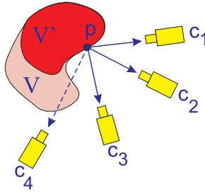
Figure 2. Illustration of the Visibility and Non-Photo-Consistency Lemmas. If  $p$  is non-photo-consistent with the photographs at  $c_1, c_2, c_3$ , it is non-photo-consistent with the entire set  $Vis_{\mathcal{V}'}(p)$ , which also includes  $c_4$ .
