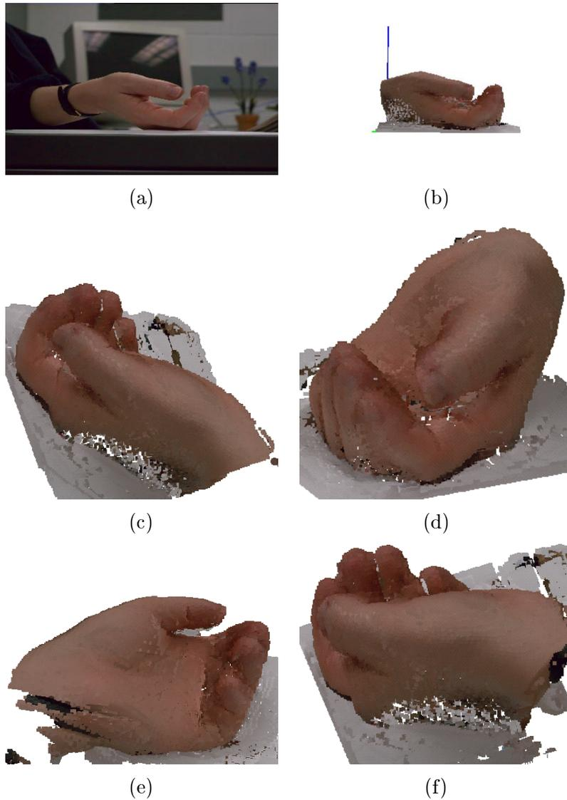
*Figure 10.* Reconstruction of a hand. An input image is shown in (a) along with views of the reconstruction from the same (b) and other (d-f) viewpoints. The reconstructed model was computed using an RGB component error threshold of 6%. The model has 112 thousand voxels and took 53 seconds to compute. The blue line in (b) indicates the z-axis of the world coordinate system.
