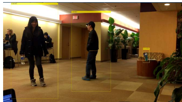
Figure 3.1.d. A poor result of HOG-people detector that recognized a bottle as a human
