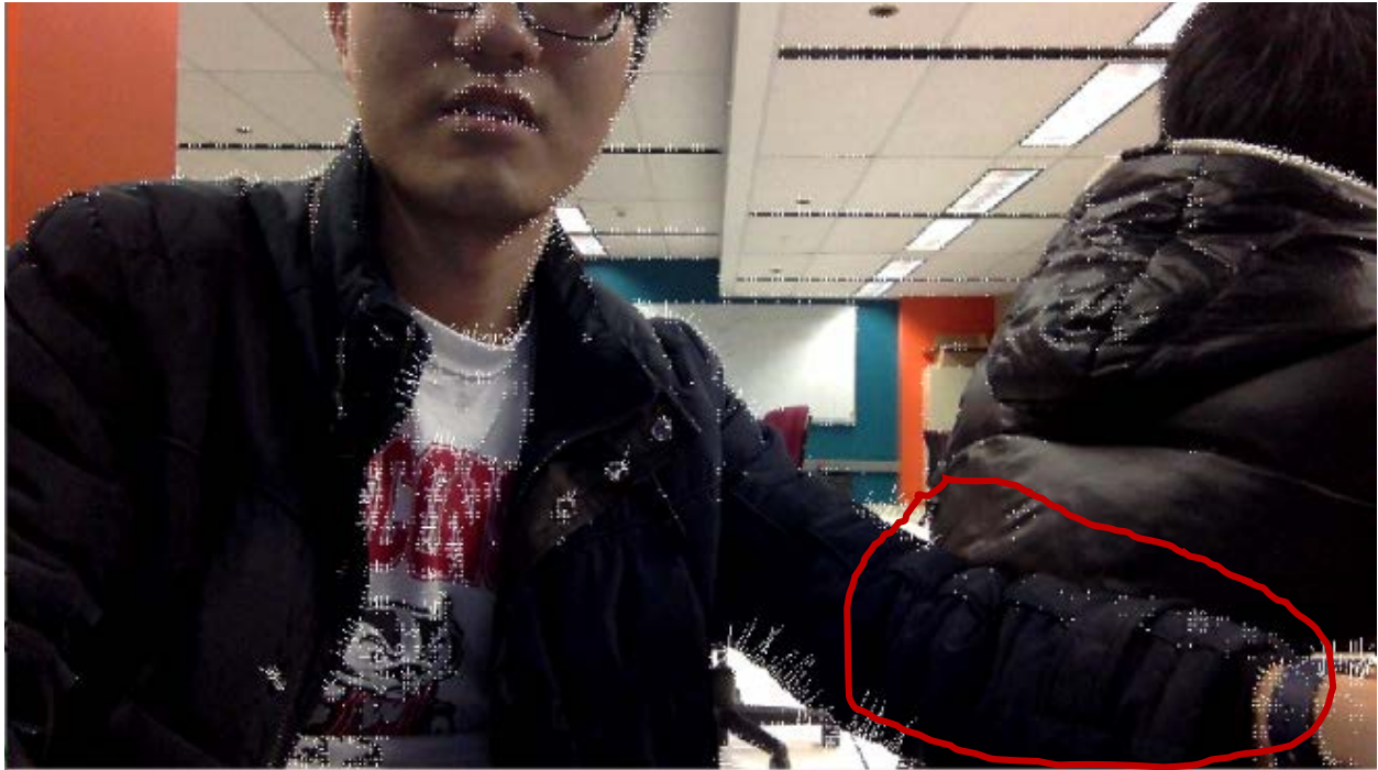
Figure 3.3.b. A poor result of Optical Flow method. On the right-hand-side of the image, the black color of the moving arm is close to the background, so the detection cannot work perfectly.
