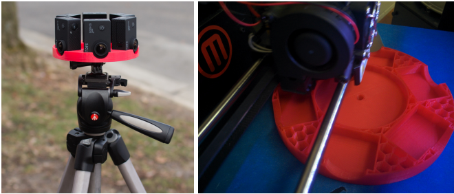
Figures 7,8: SJCAM Multi-Camera System and 3D-printed mount
