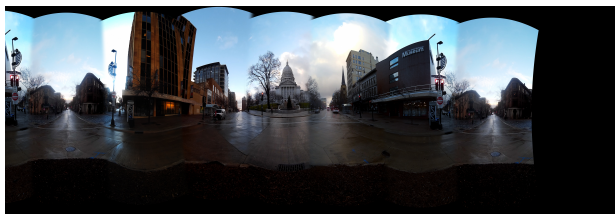
Figure 11: All six video tracks with same warping and addition pad tracks on both sides, registered and blended
