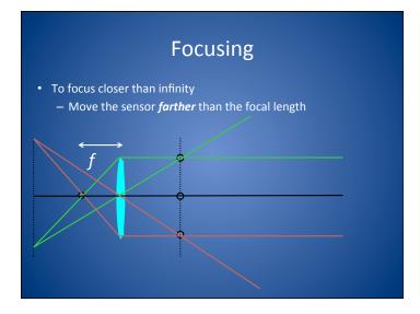
Where to Put the Sensor for an In-Focus Image?: Thin Lens Formula
